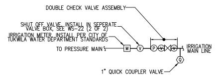
CONNECTION TO PRESSURE MAIN SHALL NOT BE MADE UNTIL IRRIGATION MAIN LINE IS PRESSURE TESTED. SEE INSTALLATION DETAIL THIS SHEET.
