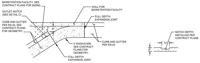
DETAIL B - OUTLET FROM BIORETENTION CURB EXTENSION
