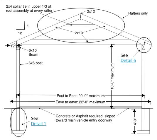
Water Diversion: Design grading to direct surface water away from the carport legs and foundation.
