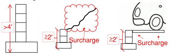
Note: All retaining walls must be properly drained; International Residential Code, Section R404.4
